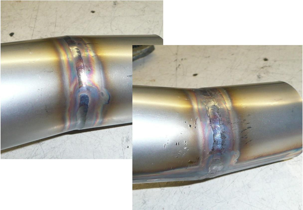
Figure 20 : Finished weld before and after hammering
