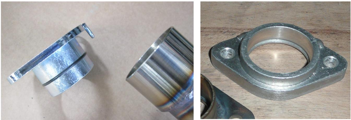
Figure 22 : Cylinder flanges with O-Ring (left: JL, right: Jolly Moto)
