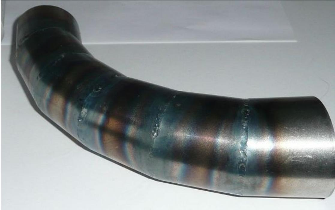
Figure 23 : Welded segments
