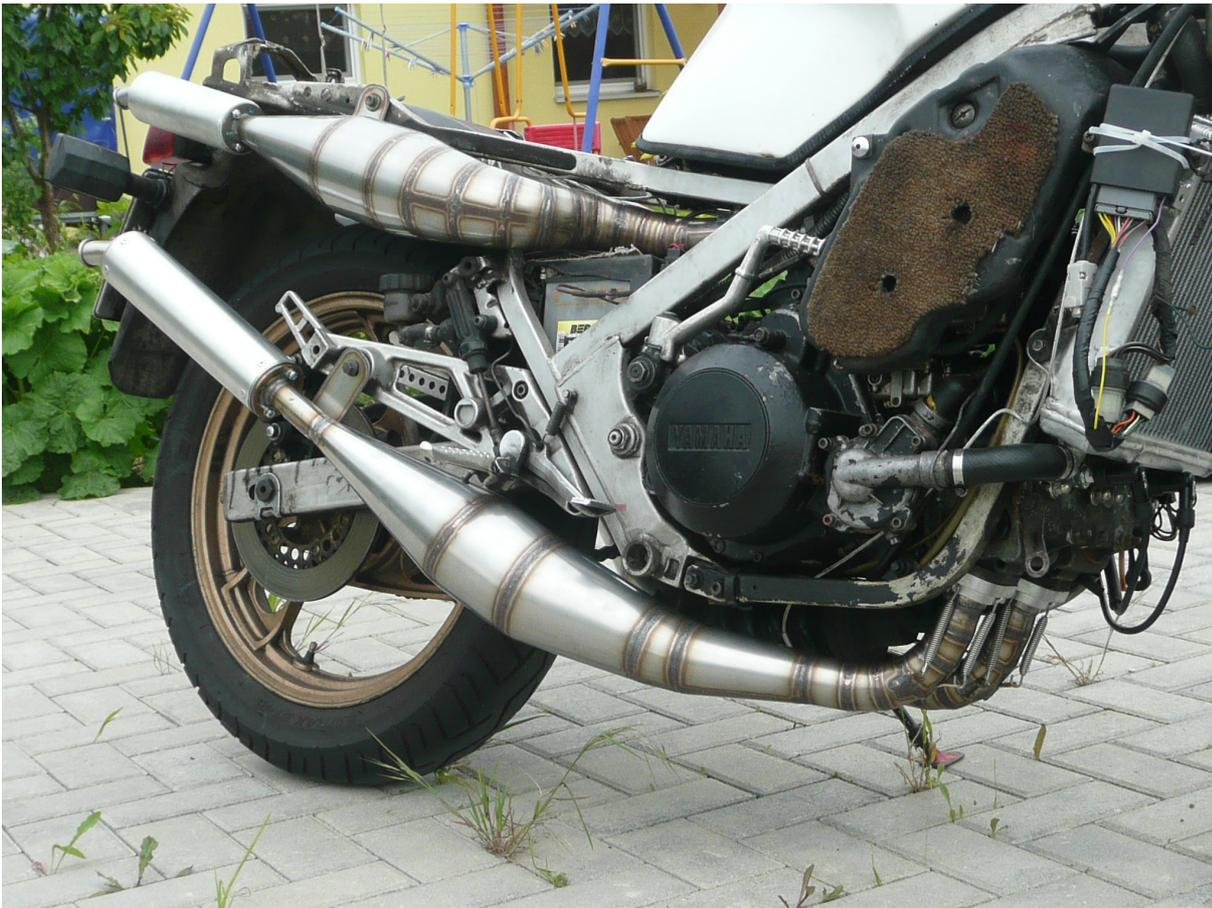
Figure 24 : RD500 DIY pipes (Design: Wayne Wright, 2013)
