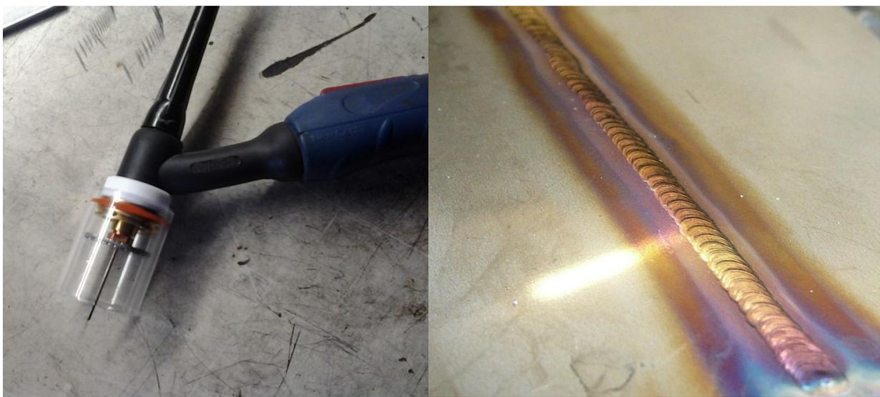
Figure 13 : Gas lens XXL and stainless test sheet
