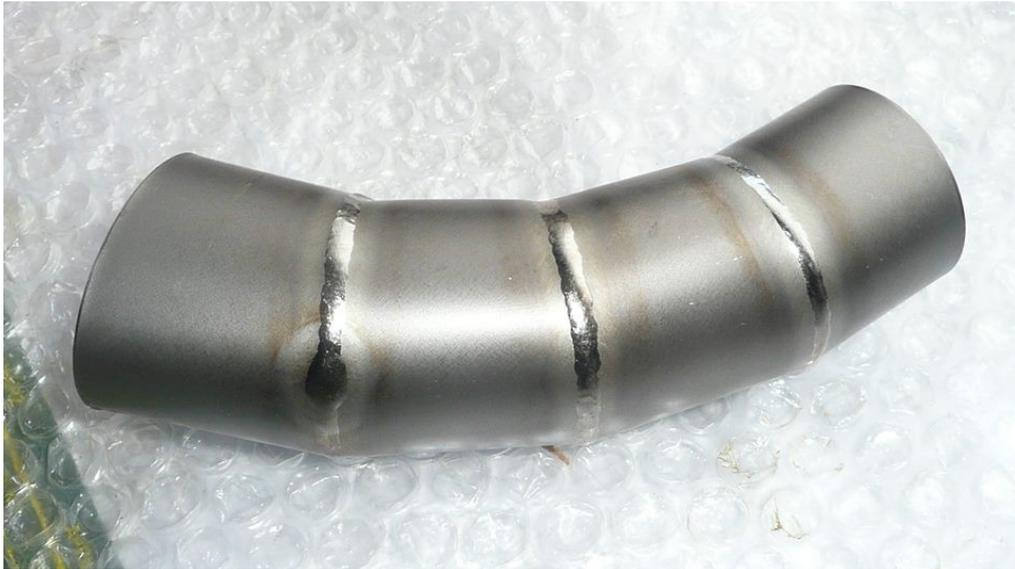
Figure 15 : Header in titanium
