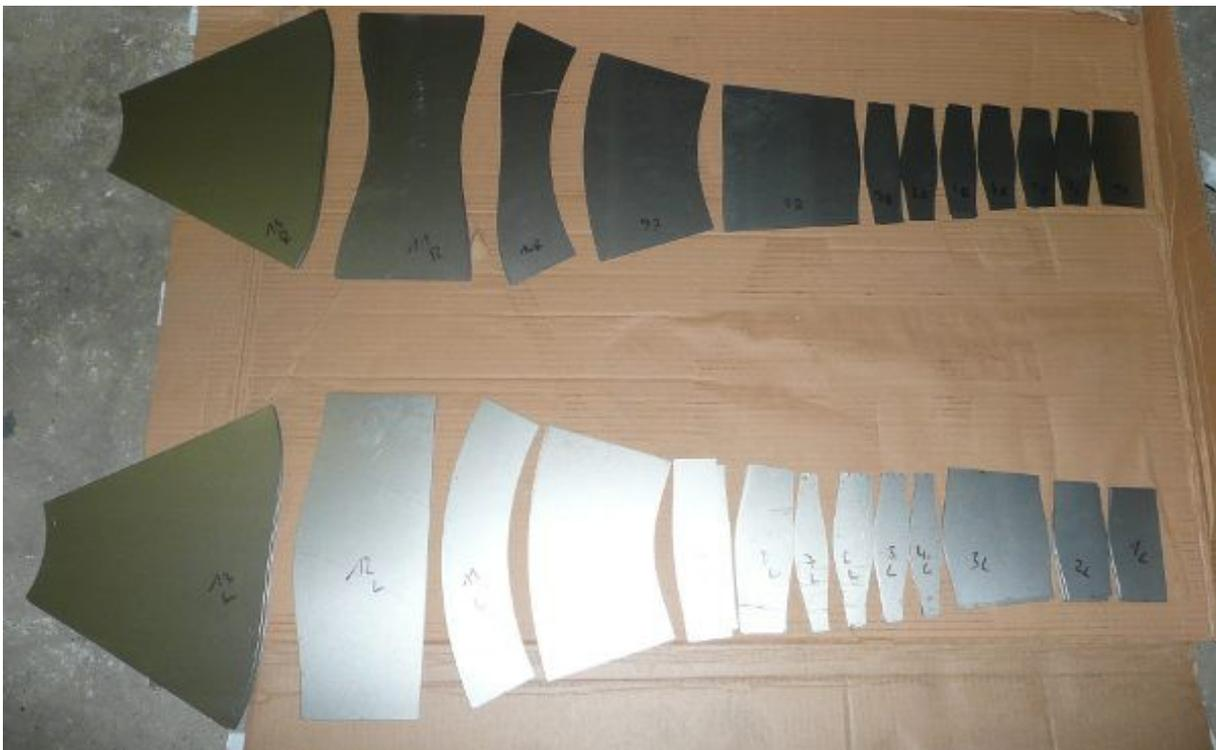
Figure 9 : Laser cut cones
