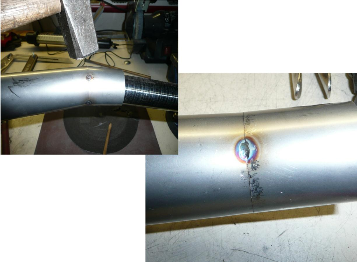
Figure 18 : Hammer after tack-weld and desired perfect (=gap-less) seam.
